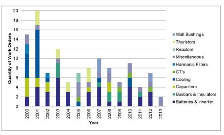
Figure 1 – SVC Suspended Failures (entire population)
