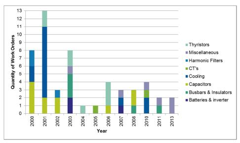
Figure 3 – KGTS SVC Suspended Failures
