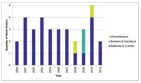
Figure 2 – HOTS SVC Suspended Failures
